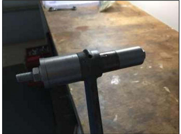
New tool installing the small end bush with a bolt. The tool can also push out the bush
